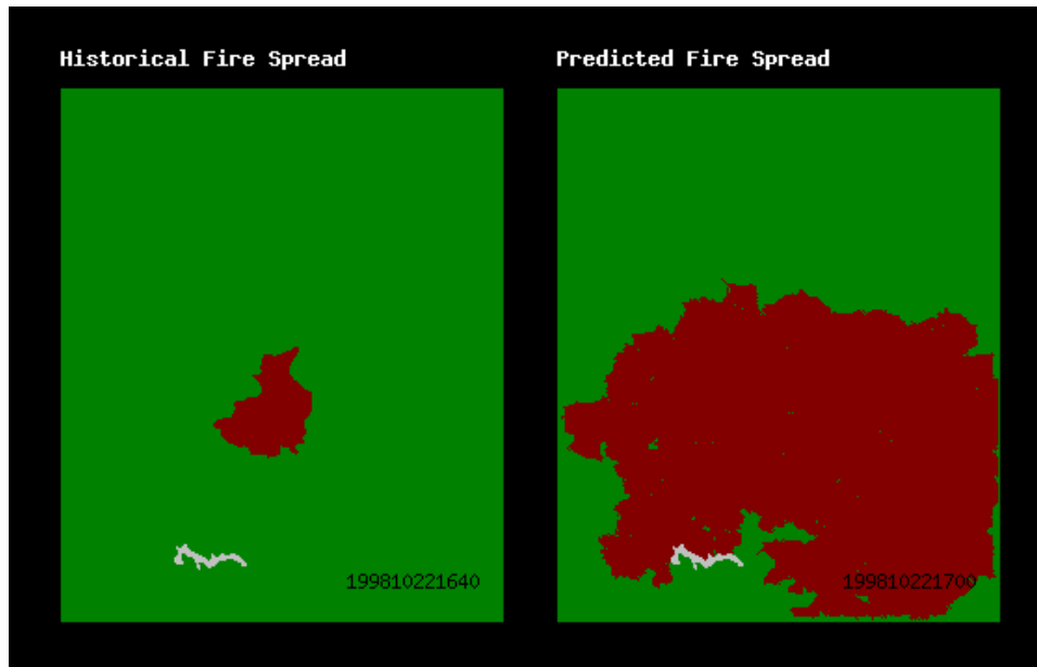
Figure 3.7. Historical (left) and predicted (right) fire behavior at 1700 hours on October 22 during the 1998 Ogilvy Fire using the HFire model. Example of severe overprediction. Inputs used during this simulation: custom fuels, and 100 meter spatial resolution.
